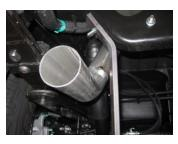
7. Install Spare tire Bracket on drivers side of Spare tire subframe as shown in the photo. Spare tire bracket will help keep the spare tire from rubbing on tailpipe. You will remove your factory spare tire heat shield. Be sure you have 1.5" clearance on all pipes near spare tire.
